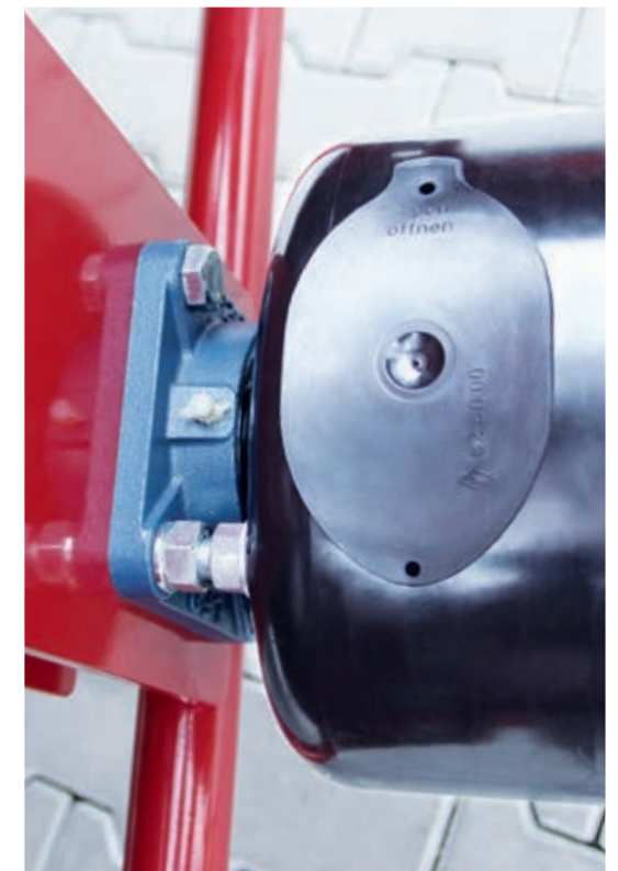
Drive of the propeller shaft of the tractor to the mixer gearbox with protective cap for the propeller shaft
