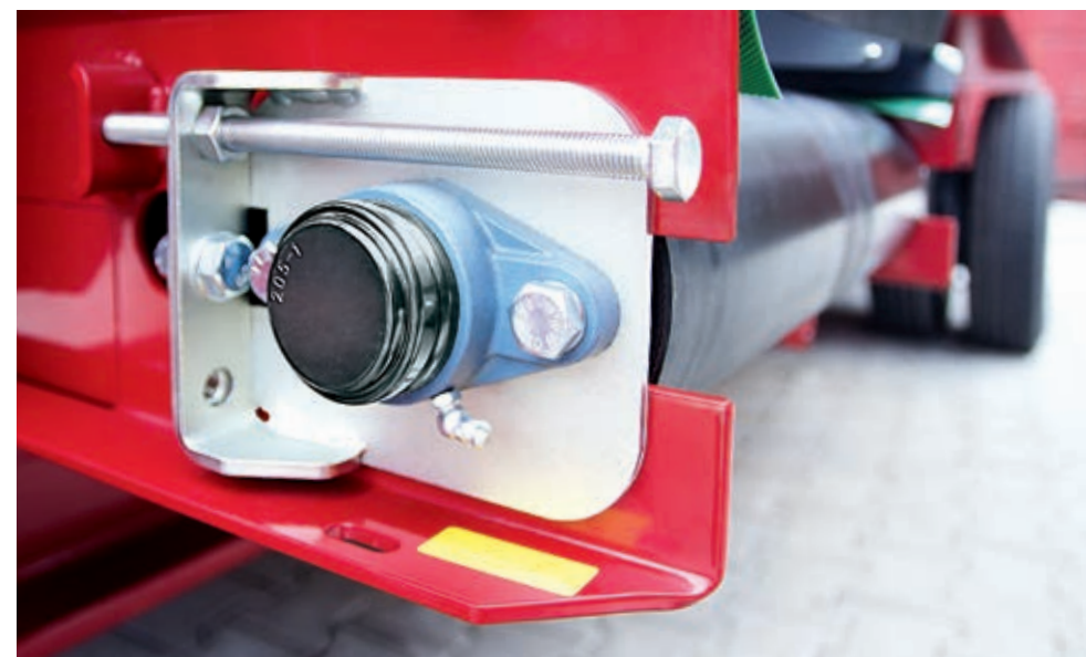
Tensioning station for the rubber belt of the conveyor, with two-hole flange bearing and protective cap
